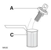
**3.** Turn the handle about  $\frac{1}{4}$  a turn anticlockwise and remove.
